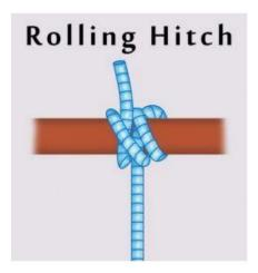
Wrap the free end of one rope around the main rope to create a Half Hitch. Make a second Half Hitch and then wrap over the entire knot to finish with a final Half Hitch to the other side from your starting place.
