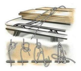
Start off by tying a Figure 8 knot with a loop of the line. Then pass the free end of the line around or through whatever you're attaching the rope to, before passing the line through the loop. Next, pull the working end tight, and secure the free end with Two Half Hitches, just below the loop.
