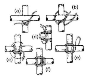
Tie a Clove Hitch to one of the poles, near the place where the two poles cross. Then wrap your line around the junction of the two poles, going under the lower pole and over the top pole. Spiral outward with these wraps five or six times. Next, wrap between the poles, biting onto the previous wrappings to tighten them. Finally, use a Square Knot to tie the free end of the rope to the free end from the Clove Hitch that started this whole lashing. Easy, right?
