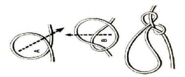
Gather some slack in the line and make a loop so part of the line runs through the middle of the loop. Grab the side of the loop and pull it through the gap between the line in the middle and the other side of the loop. Pull the new loop tight, and then pull the line to cinch the man harness knot. This knot can slip if there isn't constant tension on the newly created loop, so keep something in the loop to hold it.
