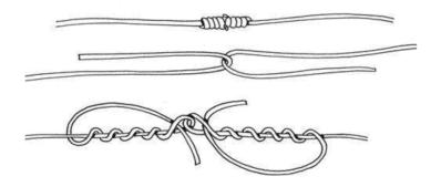
You'll start the Blood Knot by overlapping the two lines, and wrapping one free end around the other line five or six times. Pass the free end between the two lines. Wrap the other line the same number of times (five or six), and tuck the free end back between the two lines in the opposite direction of the other free end of the line. If using fishing line, spit on it to reduce friction damage.
