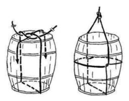
Place your barrel or other object to be lifted on top of your rope. Then tie an Overhand Knot across the top of the barrel. Open up the Overhand Knot until it wraps around the top sides of the barrel. Tie the ends of the rope together with a Square Knot and then then lift. This knot makes a fine bucket handle when the wire handle finally breaks off.
