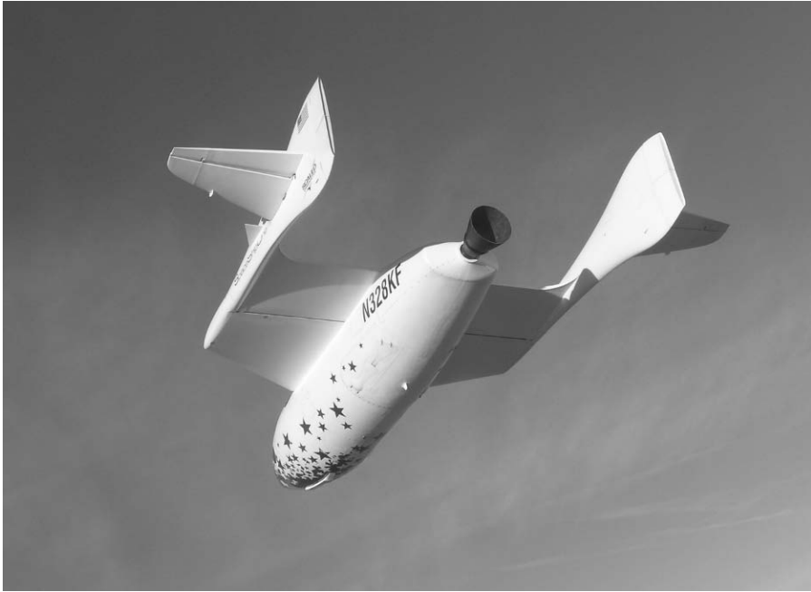
Figure 10.12: The X-prize winning SpaceShipOne on its descent after reaching in excess of a 100-km altitude in 2004. (Copyright © 2004 Mojave Aerospace Ventures LLC. Photograph by Scaled Composites. SpaceShipOne is a Paul G. Allen project.)
