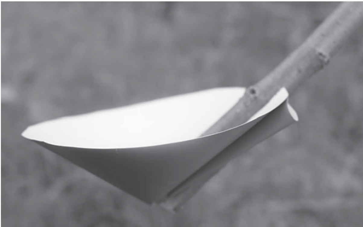
Ladle made from thin plastic material and a split stick.
