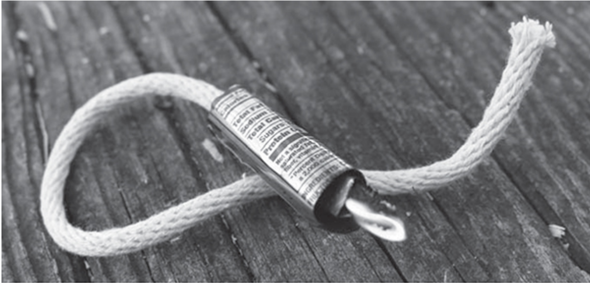
A tinder tube made from cotton rope and a rolled section of an aluminum can.
