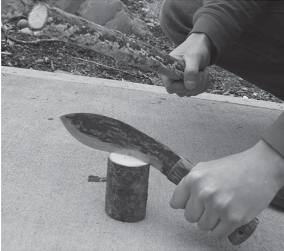
Baton position for splitting wood.
