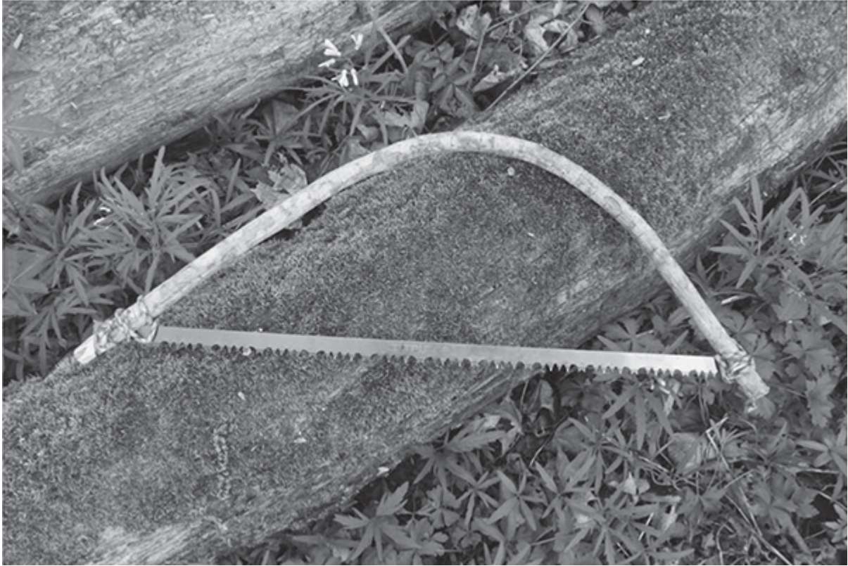
Bow saw made from a bent sapling.
