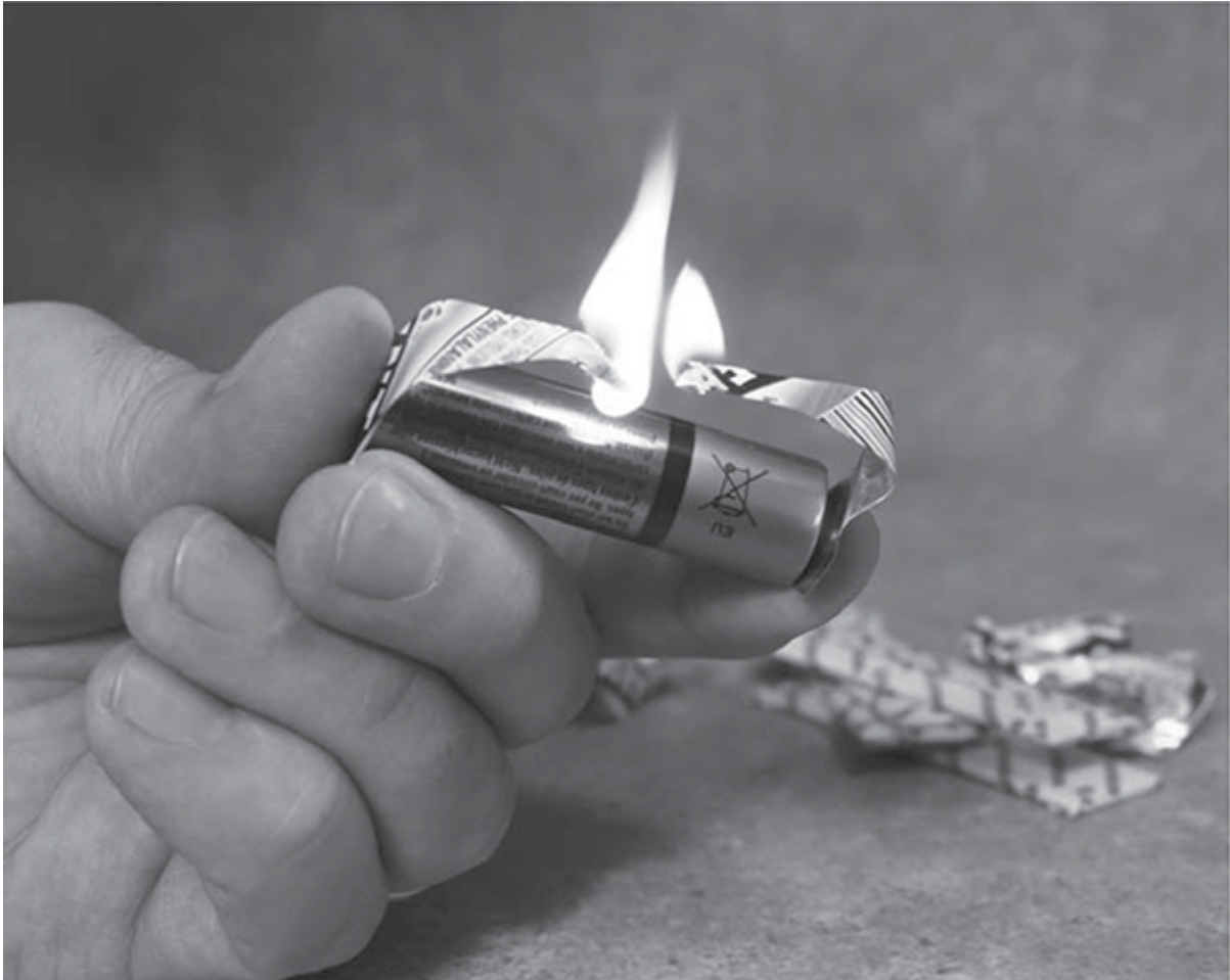
A gum wrapper bursts into flame after being used to short circuit a AA battery.
