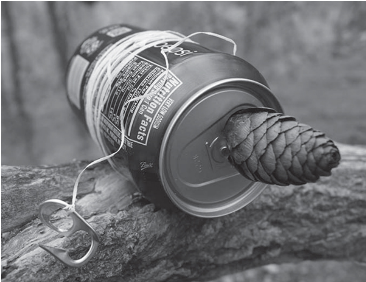
Pop can hand reel with a pull tab barbed hook.
