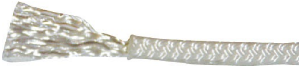
16-strand double-braided polyester cover over 16-strand braided polyester core (pictured here with exposed core)
