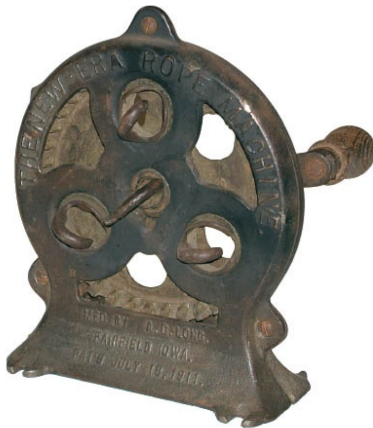
A rope-twisting machine used in World War I and during the Great Depression in Iowa, USA, to make ropes from twine and lightning conductors from wire for agricultural use.
