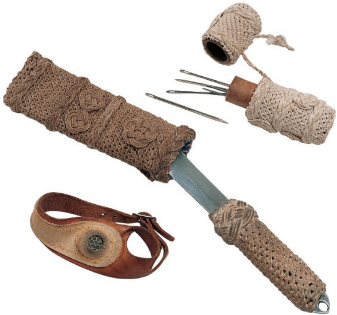
From left to right: a sailmaker's palm, sheath knife, and needle case. The sheath knife and needle case are handsomely covered with half-hitching and Turk's Head decorative ropework, collectively known as marlinespike seamanship.
