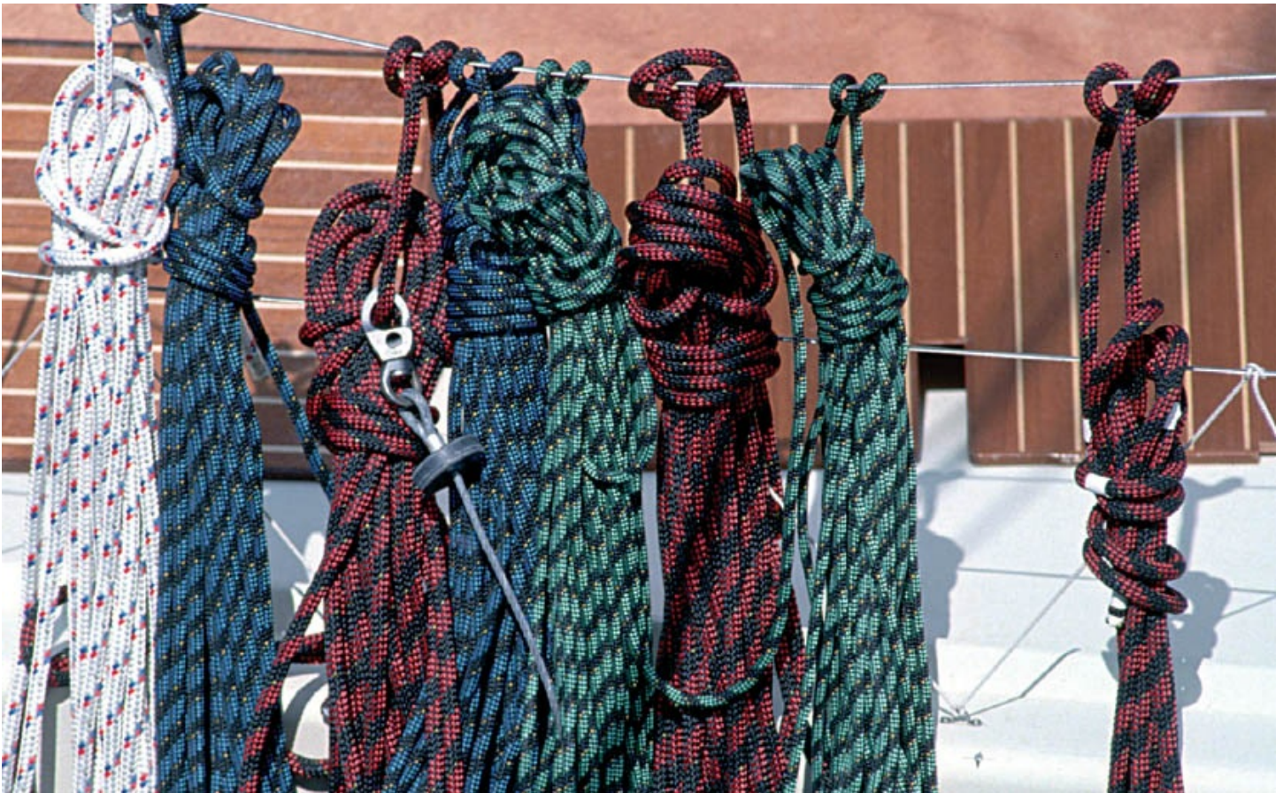
Lines hung in gasket coils dry well and are easier to locate for immediate use.
