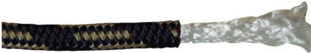
24-strand braided polyester cover over 16-strand braided multifilament polypropylene/Spectra™ core, known as Samson's XLS Extra™
