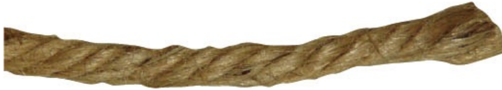
4-strand left-laid twisted hemp fibre
