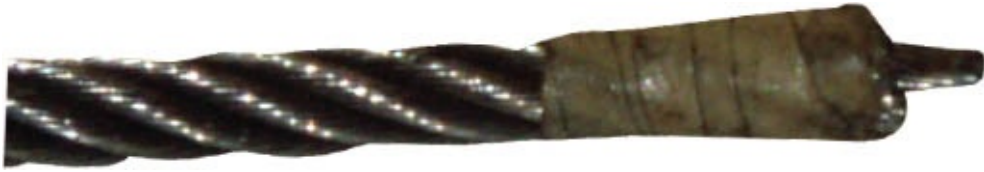
6-strand wire with Independent Wire Rope Core (6x19 IWRC), pictured here with exposed core
