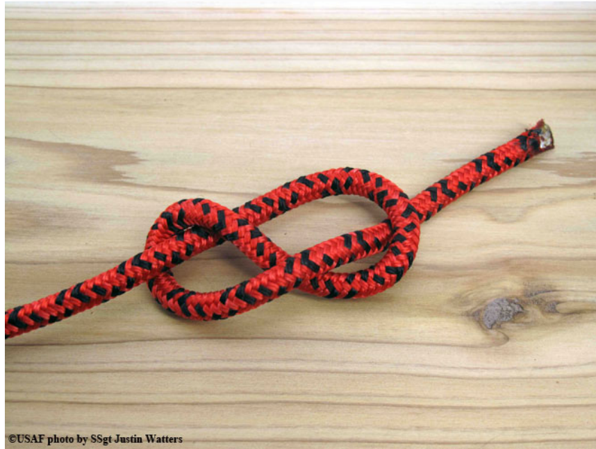
Figure 15-26 Figure-Eight Knot
