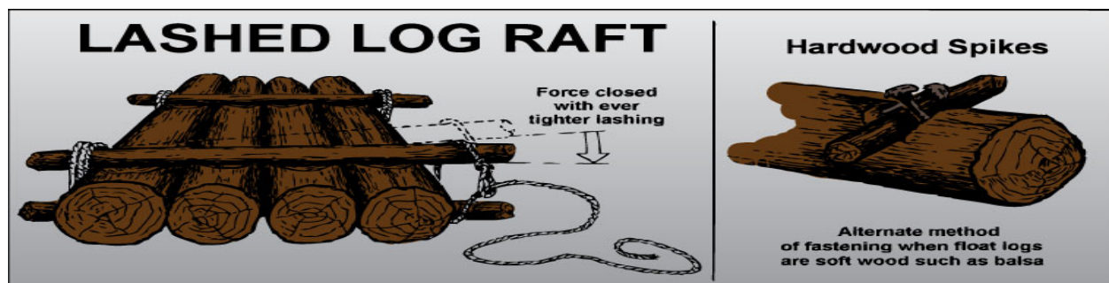
Figure 20-37 Spikes and Lashed Log Raft
